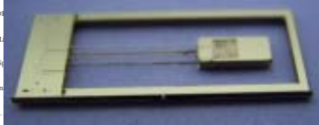
2x2 Optical MEMS Switch
