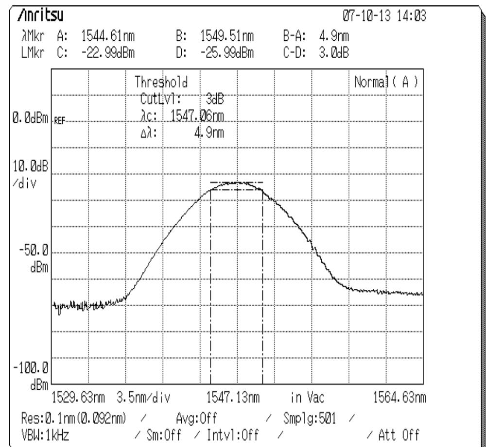
10-40GHz repetition rate, 500-800fs transform-limited pulselwidth
