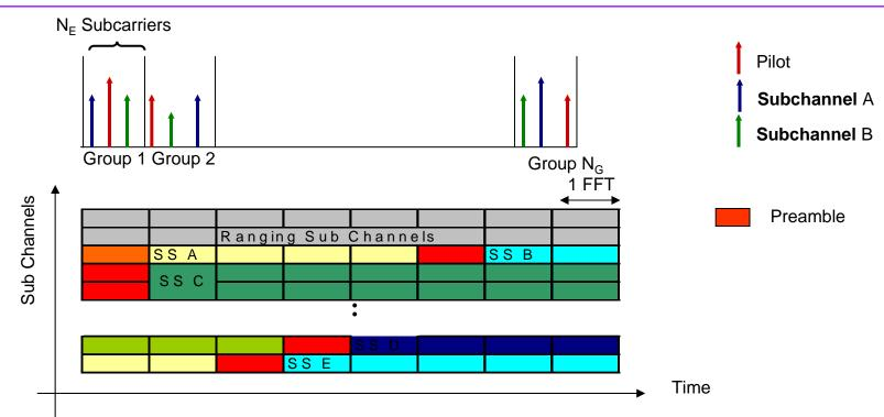
Different modulation/coding in each sub channel
