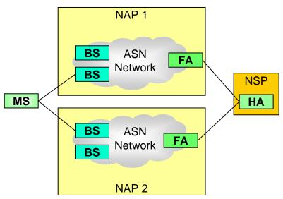
NAP: Network Access Provider NSP: Network Service Provider
